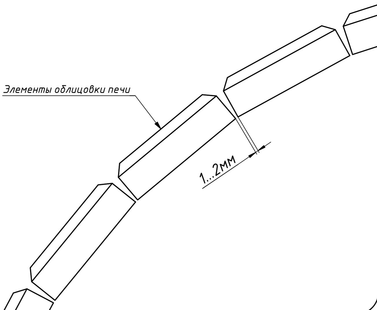
A technical line drawing of a brickwork element, likely a chimney or stove lining. It shows several rectangular bricks arranged in a staggered pattern. A specific vertical joint between two bricks in the same row is highlighted with a dimension line and the text '1...2мм', indicating the allowable vertical gap. An arrow points from the text 'Элементы облицовки печи' to the brickwork.
